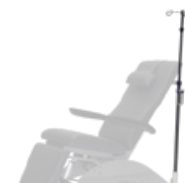
I.V. Pole stainless steel Ø 25/18 mm, one-hand height adjustable 1,070 – 1,660 mm, 4 hooks, max. 2 kg/hook, glass and holder (adapter 3082 0000 not included)
